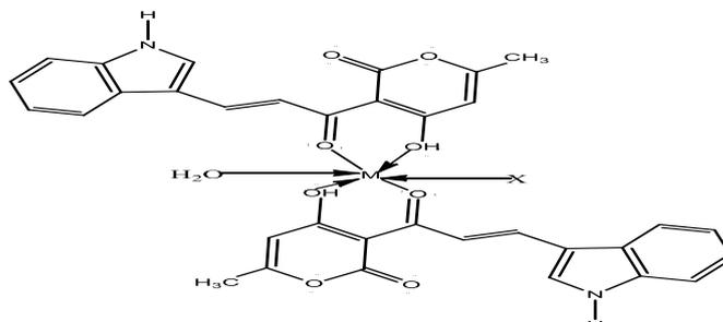
Fig. 1: Proposed structure of complex, when X= Cl, M=Fe(III) and X=H<sub>2</sub>O M=Mn(II), Co(II), Cu(II), Ni(II)
